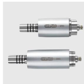
**Micromotors.** Two versions: i-MMr (3.3 Ncm) with and without LED, i-MMs (5.3 Ncm) with LED lighting and ready for endodontic treatment. Both with speed range from 100 to 40,000 rpm.
