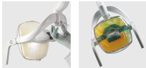
**Venus Plus L-LED.** LED operating light with hermetically sealed front screen (optional). Potentiometer-adjustable light intensity, from 3,000 to 50,000 Lux. Colour temperature 5000K. On-off control also via infrared sensor.
