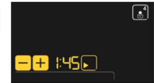
**Timer.** This function lets users keep track of application times (e.g. when etching gel or compounds are used).
