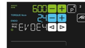
**Endo.** The i-MMs micromotor (optional) gives dentists access to all endodontic functions, which are controlled in an integrated manner by the panel on the dental unit.
