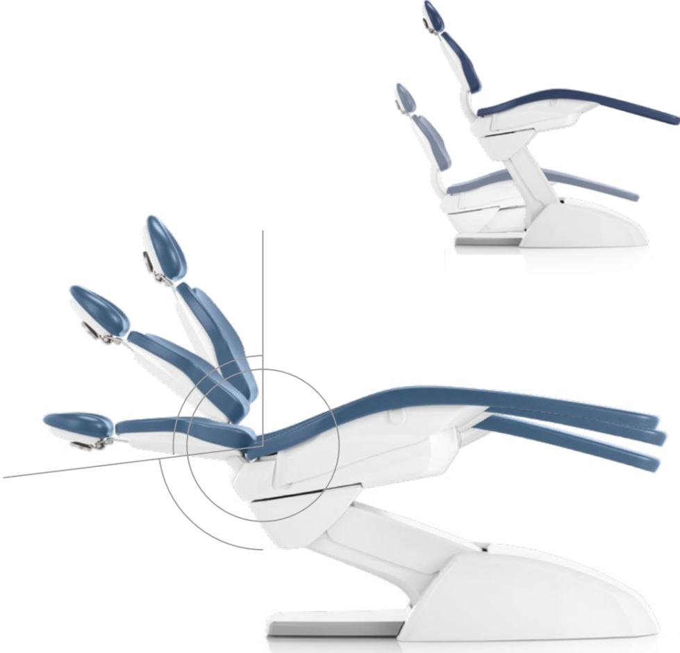
**Vertical excursion and lift capacity.** Extensive vertical travel (37-80 cm) makes it easier to provide treatment in comfort and allows easy patient chair access for the elderly. The patient chair is certified to lift patients weighing up to 190 kg.
