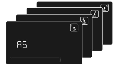
**Multi-profile feature.** Cuspidor-cup system automatisms, favourite working positions and settings for every single instrument can be saved for up to 4 different users, ensuring maximum versatility of use. This function is useful in multi-dentist surgeries or in clinics where there is high turnover of specialists.
