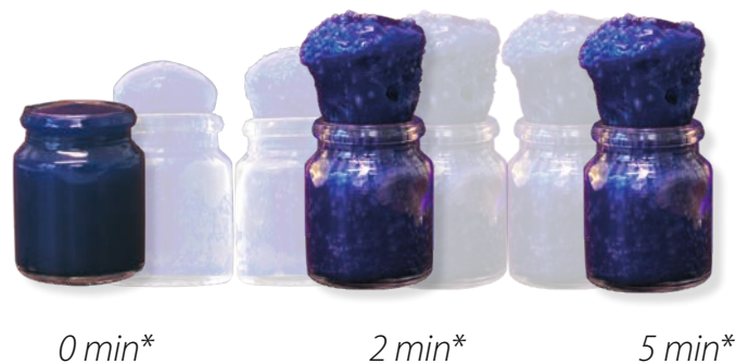
2 min*: Foaming action complete; 5 min*: Material completely cured. Total Expansion 160%
