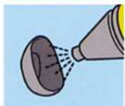
Sandblast the inner surface of the crown
