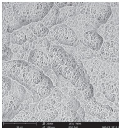
MIS C1 implant surface with micro-nano-structure (x 2,500).
