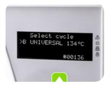
Class B cycles exclusively The Lina sterilizer works exclusively with Class B cycles and with short ECO B cycles for smaller loads.
