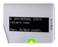
**ECO B sterilization program** The cycle time can be reduced by half for small loads.
