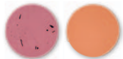
Fig. 1: Hand-mixed putty (left) compared to an automatically mixed putty material out of the Pentamix™ System from 3M ESPE (right). The automatically mixed impression material is homogeneously mixed and does not show any voids.
