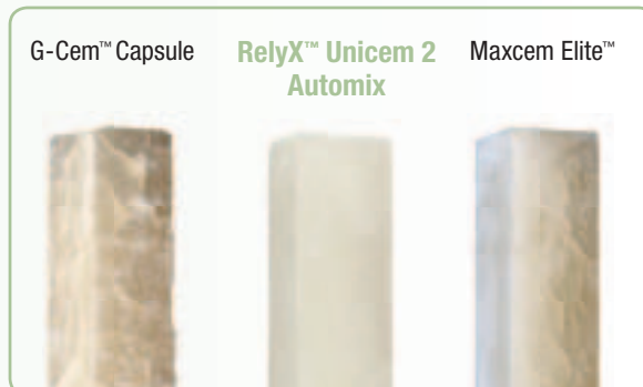
Results of stress test on self-adhesive resin cements. All samples were self-cured and thermocycled 10,000 times.
