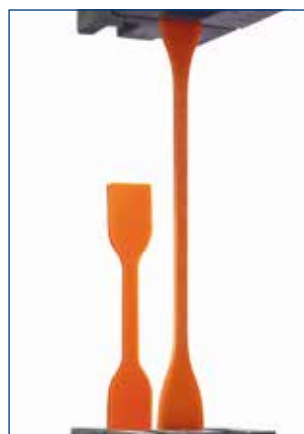
Stretching of V-Posil X-Light Fast
