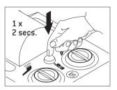
Press the program button once for about 2 seconds. Open the cover at the end of the maintenance cycle.
