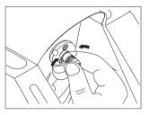
Firmly squeeze the 0-ring between thumb and forefinger and pull it off.
