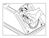
Push the appropriate adaptor onto the maintenance attachment up to the limit stop.
