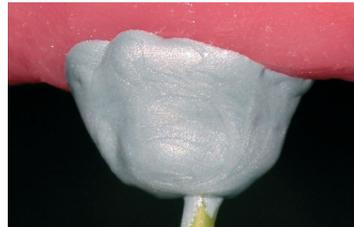
Thixotropic properties prevent slumping and dripping.
